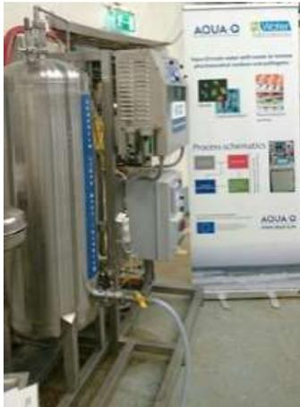
Aqua-Q has developed and composed a modular ozone polishing system and has successfully demonstrated that in a cost-effective way with a minimum dose of ozone both pharmaceutical residues and pathogens can be totally removed beyond the limit of detection.
